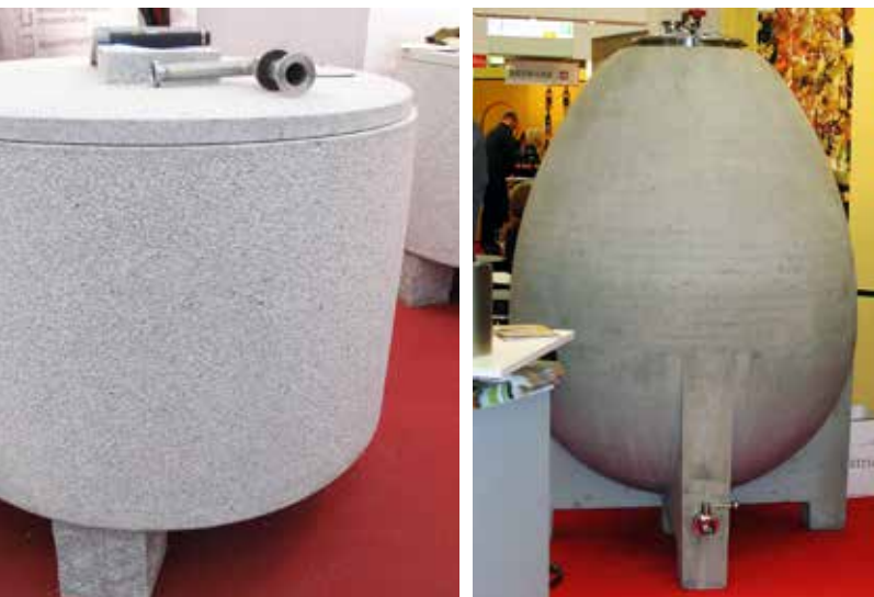
Fermenter of natural stone and Concrete egg (© Walter Kaltzin)
